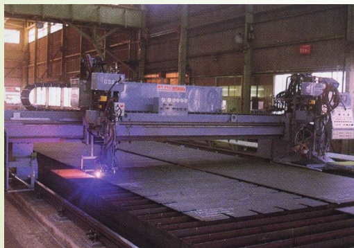
Automated Plate Cutting
