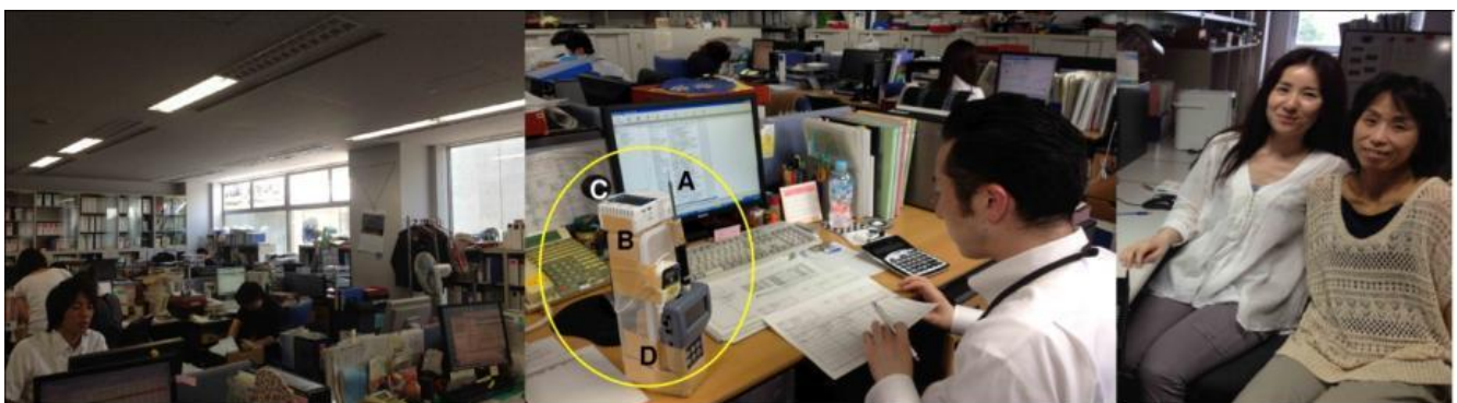
Figure 1. Typical survey environments, measurement setup and typical female clothing ensembles; (A) Omni-directional probe anemometer (Kanomax Climomaster 6531), (B) Thermo-hygro-CO 2 meter (TR-76Ui), (C) Globe thermometer (TR-52i)
