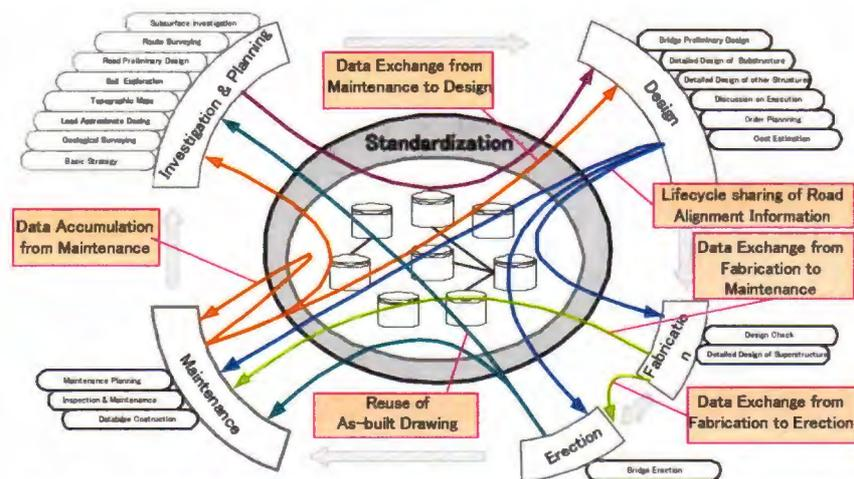
**Fig.6** Image of the ideal data sharing in each business phase of bridge construction
